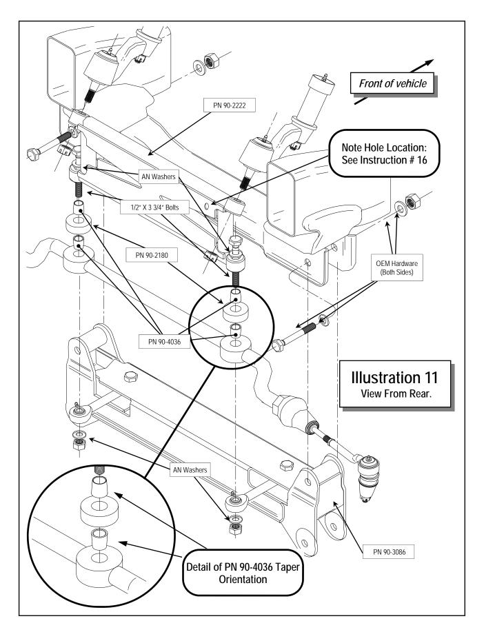
**2222)**, and rod ends from the front cross member to the center link drop using the 1/2" X 3 3/4" bolts, spacers (PN 90-2180), and reducer cones (PN 90-4036) provided. Follow the assembly shown in **ILLUSTRATION 11**. Torque the new bolts according to the torque chart on page 21 and re-torque the steering box and idler arm bolts to Manufacturers specifications.
