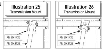
**ILLUSTRATIONS 25 & 26** as a reference. Rotate the strut up to the transmission cross member and test fit the mounts until a satisfactory location is found. After you have located the position of the holes, drill them out with a 1/2" drill bit and install the saddles (PN 90-1435) with the supplied 1/2" X 1 1/4"
