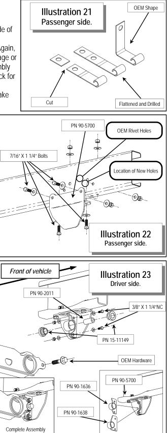
same orientation that they were removed (i.e. left front to left front, right front to right front!). *Reset the torsion bar preload bolts using the measurements previously taken.*
