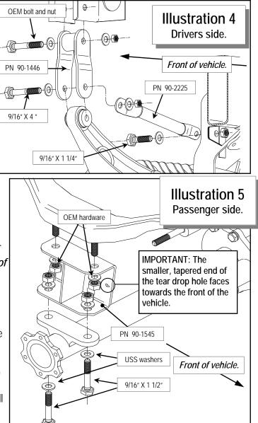
tighten the assembly enough so that the strut can be moved without much effort to complete *step 6*.
