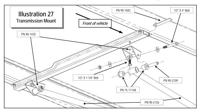
bolts, washers, and tab nuts. See **ILLUSTRATIONS 24, 26, & 27**. Rotate the struts back up and install the **1/2**" **X 4**" bolts supplied. Repeat this procedure for the other side. Torque the compression strut hardware to specifications.
