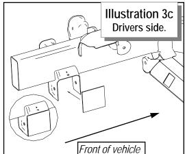
the frame rail. The driver side front drop uses the OEM power steering bolt. Clamp each drop firmly to the frame and using the drops as a guide, drill pilot holes. Remove the drop and finish drilling with a 1/2" drill bit. Repeat this for the three remaining drops. DO NOT BOLT ON AT THIS TIME. See **ILLUSTRATIONS** 12, 13, 14, & 15.
