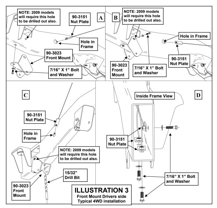
ing the front mount as a template center punch and drill out the remaining lower rear hole using a **15/32**" drill bit. See ILLUSTRATION 3C.
