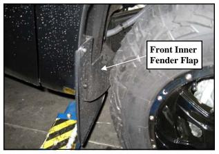
2. Remove the front flap. Push the inner fender forward to create additional clearance. The mounting location on the inner fender will need to be trimmed to create the additional clearance. The inner mounting hole will also have to be redrilled in it's new position.
