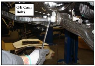
6. Unbolt the sway bar end links from the lower control arm. Save the hardware for reuse.
