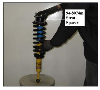
13.Install the strut assembly into the strut tower and secure using the upper (4) 10mm flange nuts. (Make
