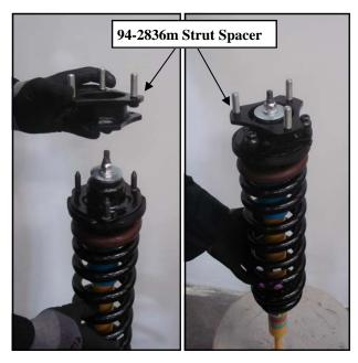
11. Install the strut assembly into the strut tower and secure using the upper (3) 10mm flange nuts. (Make sure the bottom of the strut is aligned properly)
