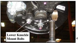
6. Loosen, but **DO NOT** remove, the lower control arm cam bolts.
