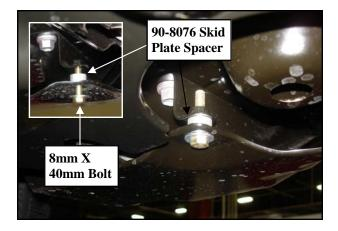
20.Reinstall the differential skid plate if previously removed from the vehicle, using the supplied 8mm X 40mm bolts, 5/16" washers and spacers (90-8076).
