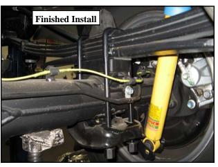
8. Secure the assembly with the **U-bolts** (13-90126Em) and new hi-nuts and washers from hardware pack (20-65303m). Do not torque the **U-bolts** at this time.
