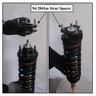
12.Install the strut assembly into the strut tower and secure using the upper (3) 10mm flange nuts. (Make sure the bottom of the strut is aligned properly)
