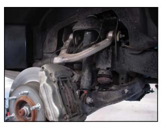
5. Now would also be a good time to inspect the shocks for damage or fluid leakage. Replace if necessary.
