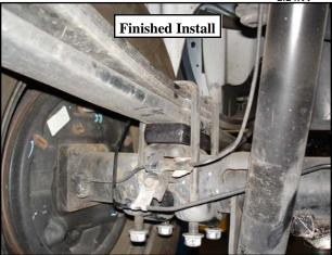
Secure the assembly with the **U-bolts** (13-90086Em) and new hi-nuts and washers from hardware pack (20-65303m). Do not torque the **U-bolts** at this time.
