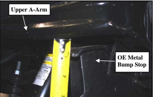
13. Now would also be a good time to inspect the shocks for damage or fluid leakage. Replace if necessary.
