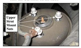
NOTE: Because this kit retains the use of the OE studs the vehicle can easily be returned to it's stock form.
