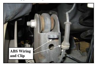
4. Unclip the ABS lines from the clips from the frame rails.
