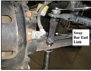
9. Support the lower control arm with a jack and unbolt the lower strut mounting bolts from the lower control arm mount.
