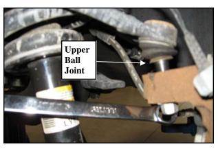
8. Unbolt and remove the sway bar end links from the vehicle.
