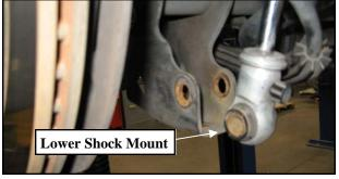
11. Lower the rear axle enough to remove the coil springs from the front spring pockets. Save the factory isolators for re-use.
