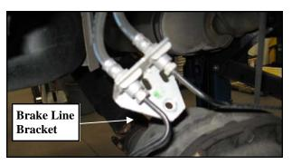
7. Unbolt the hard brake line brackets from the rear axle. Save the hardware for reuse.
