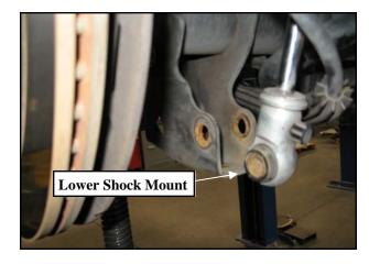
12. Lower the rear axle enough to remove the coil springs from the front spring pockets. Save the factory isolators for re-use.
