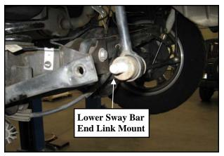
11. Unbolt the lower shock mount bolts on both sides of the vehicle. It may be necessary that you slightly raise the axle to unload the shocks for removal.
