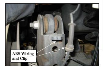
5. Unclip the ABS lines from the clips from the frame rails.
