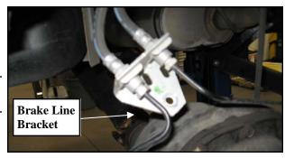
8. Unbolt the hard brake line brackets from the rear axle. Save the hardware for reuse.
