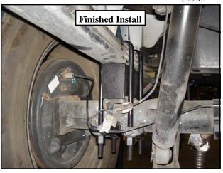
8. Secure the assembly with the **U-bolts** (13-90086Em) and new hi-nuts and washers from hardware pack (20-65303m). Do not torque the **U-bolts** at this time.
