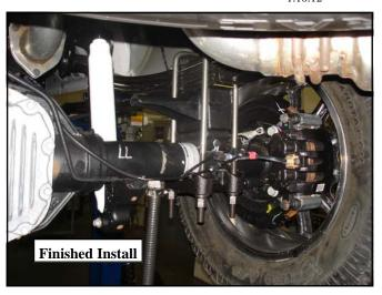
drvr and 95-503SD pass). Make sure the pin fits into the hole on the spring perch. Use your floor jack to raise the axle to the spring making sure the pin on the leaf spring assembly fits into the hole on the lift block. Secure the assembly with the supplied U-bolts (13-90560Em) and hardware (20-65472m). Do not torque the nuts at this time.
