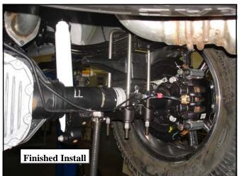
drvr and 95-403SD pass). Make sure the pin fits into the hole on the spring perch. Use your floor jack to raise the axle to the spring making sure the pin on the leaf spring assembly fits into the hole on the lift block. Secure the assembly with the supplied U-bolts (13-90540Em) and hardware (20-65472m). Do not torque the nuts at this time.
