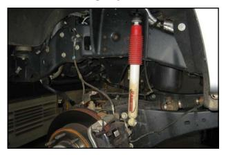
Compress spring down, install new coil spacer (94-2859), poly ring (90-4198), OE spring isolator and reinstall spring. Be sure to line up the previously applied coil spring reference mark.
