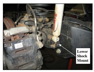
6. Disconnect the end links to the sway bar, frame brake line bracket and **OE** shocks. (both sides).
