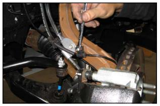
Unbolt the upper ball joint nut, but <u>DO NOT</u> remove it from the knuckle. Separate using the appropriate tool.
