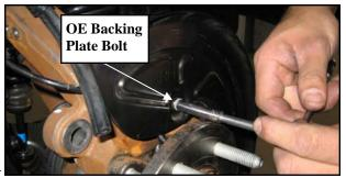
13. Unbolt the ABS sensor from the hub. Remove the CV axle end nut. Save for reinstallation.
