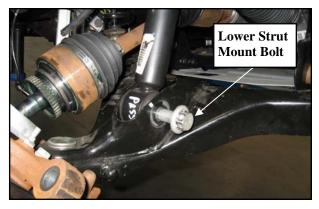
11. Support the lower control arm with a floor
