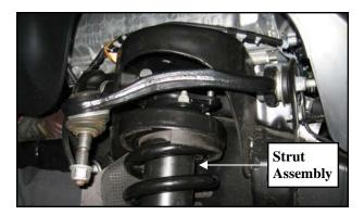
22. Install the lower strut bolt in the original position and torque to manufacturers specifica-
