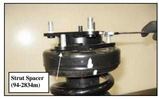
16. Install the strut assembly into the strut tower and start the (3) upper 10mm flange nuts.
