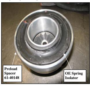
17. Reinstall the compressed coil spring onto the strut assembly using the reference marks as a guide.
