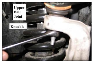
9. Support the lower control arm with a jack and unbolt the lower strut mounting bolts from the lower control arm mount.
