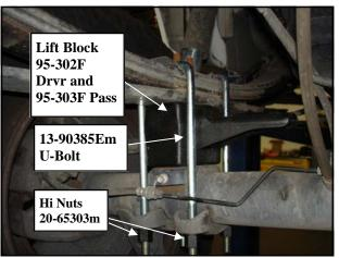
Secure the assembly with the U-bolts (13-90385Em) and new hi-nuts and washers from hardware pack (20-65303m). Do not torque the U-bolts at this time.
