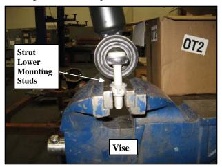
23. With the strut leaning opposite the pulling direction, carefully pull the top of the strut assembly to rotate it on the lower mount until it reaches an equal but opposite angle leaning toward you.
