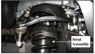
25. Install the lower strut bolt in the original position and torque to manufacturers specifications.
