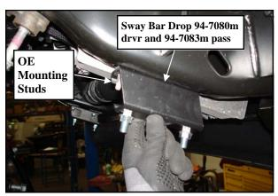
16. Carefully raise the sway bar back into place and secure the supplied hardware from pack (90-6340m).
