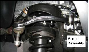
19. Install the lower strut bolt in the original position and torque to manufacturers specifications.
