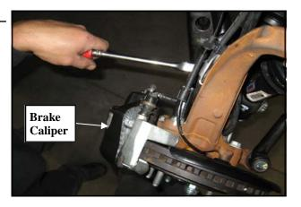
10. Remove the front rotors from the front hub.
