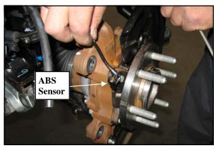
12. Unbolt the ABS sensor from the hub.
