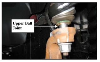
remove it from the knuckle. Separate using the appropriate tool.
