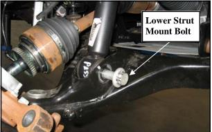
control arm. Save the hardware for reinstallation. Be sure to note the direction of the bolt for reinstallation.
