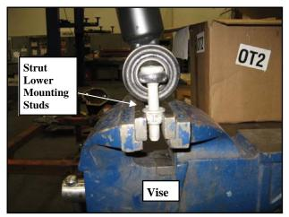
to be repositioned in order to properly align them with the lower control arms.
