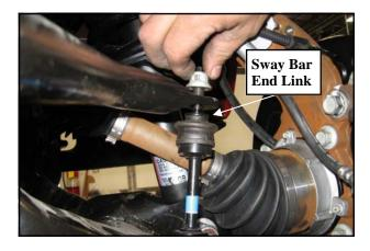
13. Unbolt the sway bar from the sway bar end links. Save hardware for reinstallation.
