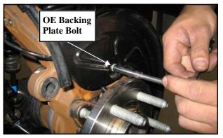
11. Remove the backing plate bolt from the knuckle to access the ABS sensor.
