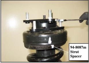
previously removed **OE** nuts. Torque the nuts to factory specifications. *NOTE: Be sure to use thread locker on*
