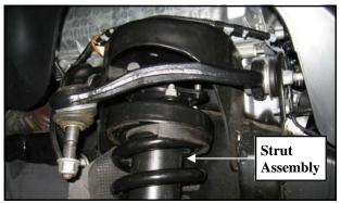
aligned as well) Torque the upper strut tower 10mm nuts to 60 ft./lbs.
