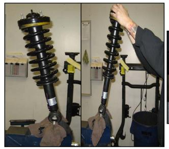
direction, carefully pull the top of the strut assembly to rotate it on the lower mount until it reaches an equal but opposite angle leaning toward you.
