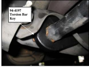
IMPORTANT! Make sure Torsion Bar is extended at least <sup>1</sup>/4" inch through the Torsion Key.
