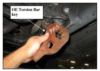
8. Install the Pro Comp Forged torsion key (94-4197) and slide the torsion bar back into position. Be sure to line up the previously applied orientation marks.
