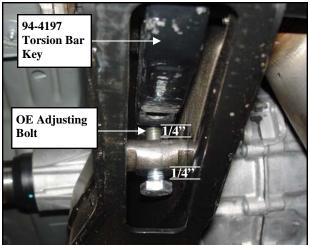
NOTE: Each <sup>1</sup>/<sub>4</sub>" of adjustment on the bolt equals approximately 1" at the wheel.
