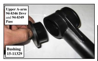
15.Insert the sleeve (90-8222) into the upper A-arm bushings.
