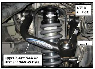
IMPORTANT!: When the 1/2" upper ball joint bolt is properly tightened there will be a 1/16" gap between the OE knuckle and the bottom spacer (90-4622).
