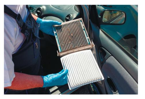
More than 90% of new cars and trucks have cabin air filters, but many drivers don't know it. Cabin filters are usually behind the dashboard or under the windshield and not always the easiest to find. We've grown up checking the air filter at each oil change, but not the cabin filter. Cabin air filters didn't start showing up in cars until the late 1980's.
