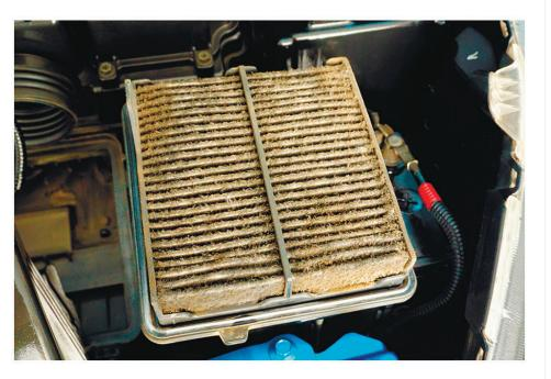
A clean air filter protects the engine from harmful debris without obstructing airflow. To promote engine health, most automotive manufacturers recommend replacing the air filter every 15,000 to 30,000 miles. But, does replacing your car's air filter also improve gas mileage?
