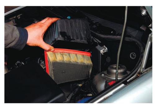
An air filter is like a security guard for your engine. It keeps the undesirables (dirt and debris) out while letting power-producing air in. A restricted air filter can cause many problems, including an illuminated check engine light.
