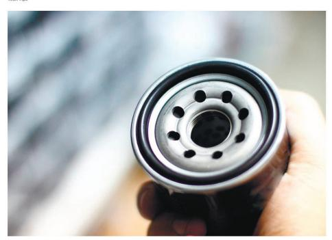
In layman's terms, the pressurized oil inside the engine enters the oil filter via the holes located in the base plate of the filter.
