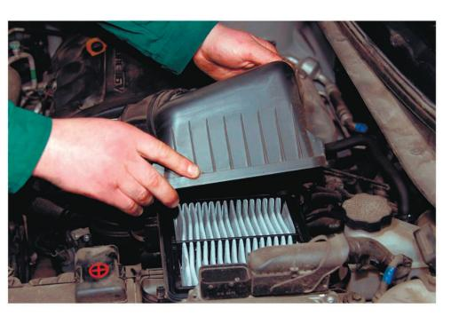
The air filter keeps dirt and debris from entering the engine. Most air filters are made from a combination of paper and synthetic fibers that trap harmful particles. Without a functional air filter, dirt and debris can sneak into the engine, which can have a number of costly consequences.
