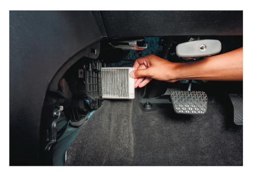
Cabin filters prevent harmful dirt and debris from entering your vehicle's interior. But did you know they also protect your car's heating, ventilation, and air conditioning (HVAC) system? Cabin filters are nearly as important to your vehicle's health as they are to your own.
