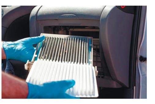
Cabin air filters are found on most late model vehicles. They clean the air that comes into the cabin through the ventilation, heating and cooling systems. The filter catches small particles such as pollen, dust, and other airborne materials, so they don't enter the cabin. A person that has allergies or respiratory problems can benefit greatly from having this type of filtration system.
