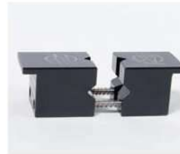
These V-Jaws are a must for any shock builder. Holds the shock shaft horizontally or vertically up to 16mm/.625" diameter. Spring loaded so they will stay in the vise when not in use.
