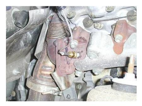
We chose to drill a 21/64" hole and tap it for a port in the 1/8" NPT the exhaust manifold for a more accurate exhaust temperature reading. A turbocharger can absorb anywhere between 100° and 300° F, depending on the engine RPM and load, as the exhaust heat turns into mechanical energy and spins the turbine.
