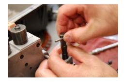
**Step 9**Install the tube after Accumulators and Solenoid Brackets. (1x long gold bolt)
