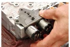
**Step 7** Place link into the valve groove.
