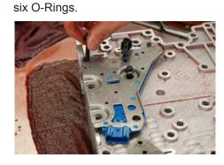
**Step 8**Slide the Valve into VB to hold in place.
