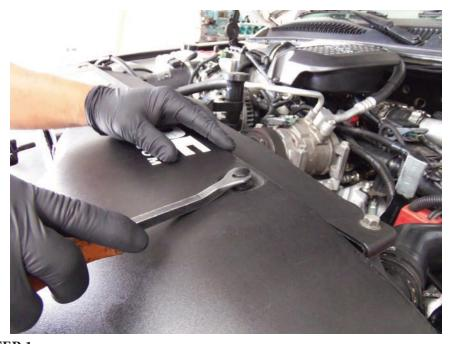
**STEP 1**Remove retaining clips and radiator cover.
