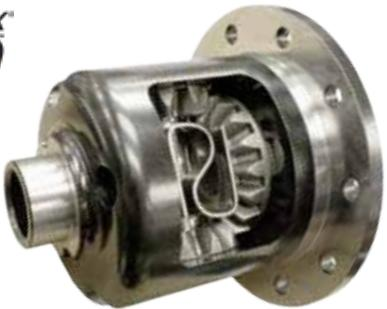
The Powertrax Grip LS, is a [clutch type differential](#) in a forged steel case. This differential uses a set of carbon clutch discs to provide traction as needed, is rebuildable and serviceable, and aimed squarely at the street machine market.
