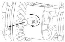
**38.** Using the retaining bolt as a handle, insert the shaft into the differential. Press hard while twisting to pass shaft by springs.
