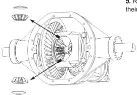
9. Remove both spider gears and their thrust washers.
