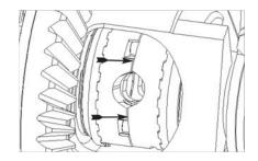
**24.** Wedge both drivers in engagement with couplers. Rotate driver's side wheel forward 1/4 turn to reveal spring slot.
