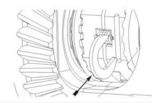
**35.** Making sure drivers stay engaged with couplers, carefully rotate both wheels backwards 1/4 turn to expose pinion shaft opening.
