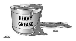
**13.** Apply wheel bearing grease to saddle springs and seat in holes.
