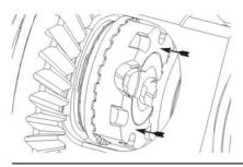
**19.** Verify spacer paddle is aligned with paddle opening in synchro ring and press driver/spacer down onto coupler. Driver teeth should be fully engaged all the way around.
