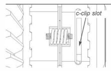
**33.** Making sure drivers stay engaged with couplers, carefully rotate wheels until c-clip slot is accessible. Verify c-clip groove on axle is accessible through c-clip slots on driver and spacer.
