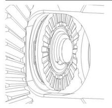
**15.** Install c-clip on ring gear side axle shaft only.
