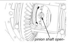
**36.** Feel through pinion shaft opening and verify both spacers and drivers are fully seated onto couplers. Press down on thrust slugs so that they are seated against the axle ends. Verify all 8 saddle springs are fully seated in holes.
