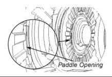
17. Insert the thrust slug into the non-slotted spacer. Insert the non-slotted spacer/thrust slug into the non-slotted driver. Seat the spacer paddle at the paddle opening in driver (missing extended tooth).
