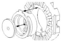
**20.** Insert the thrust slug into the slotted spacer. Insert the slotted spacer/thrust slug into the slotted driver. Seat the spacer paddle at the paddle opening in driver (missing extended tooth).
