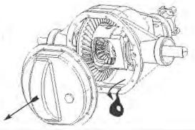
7. Expose pinion shaft; remove retaining bolt/roll pin and shaft.
