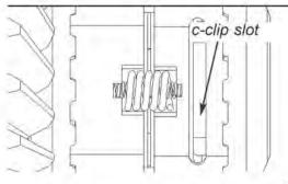
**33.** Making sure drivers stay engaged with couplers, carefully rotate wheels until c-clip slot is accessible. Verify c-clip groove on axle is accessible through c-clip slots on driver and spacer. **34.** Insert 2nd c-clip through c-clip slot in driver onto axle shaft; pull axle shaft out to seat c-clip.
