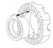
**18.** Insert driver/spacer as shown, making sure spacer paddle is facing out towards you.
