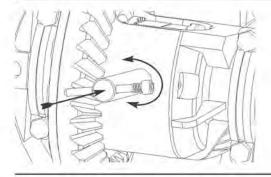
**38.** Using the retaining bolt/roll-pin as a handle, insert the shaft into the differential. Press hard while twisting to pass shaft by springs.
