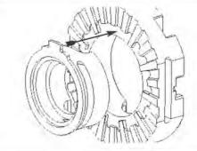
**20.** Insert the slotted spacer into the slotted driver. Seat the spacer paddle at the paddle opening in driver (missing extended tooth).
