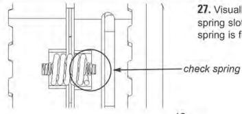
**27.** Visually inspect notches in spring slot to make sure inner spring is fully seated.
