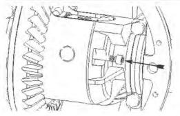
**39.** Insert retaining bolt/roll-pin into case/shaft. Tighten retaining bolt firmly.
