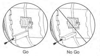
**31.** Check the gap between drivers using check block. The narrow side of the block should fit between the drivers, but the wider side should not fit.
