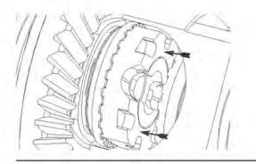
**19.** Verify spacer paddle is aligned with paddle opening in synchro ring and press driver/spacer down onto coupler. Driver teeth should be fully engaged all the way around.
