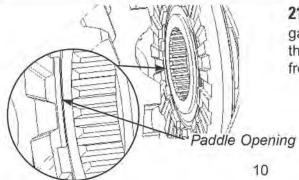
**21.** Verify paddle opening (widest gap) in other synchro ring is facing the back of the differential, away from you.
