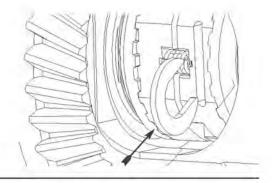
**35.** Making sure drivers stay engaged with couplers, carefully rotate both wheels backwards 1/4 turn to expose pinion shaft opening.
