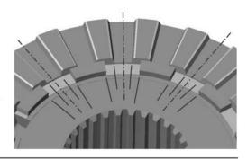
**18.** Apply wheel bearing grease to driver teeth.
