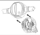
**8.** Mark the position and orientation of the bearing caps to the third member and bearing adjusters to the adjuster locks. *These parts are not interchangeable and must be reinstalled in their original positions.*
