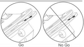
**25.** If the gap is correct, remove the cap, gage ring, and coupler to proceed.
