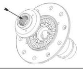
**31.** Install the cap onto the differential case. *Make sure the two case halves line up to their original positions.*
