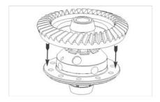
**32.** Reinstall the ring gear back onto the case. *Make sure the mark on the ring gear lines up with the mark on the two halves of the case.*
