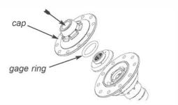
**24.** Check the gap in the differential case using the gage block. The narrow side of the gage block should fit in the gap, but the wider side should not fit.
