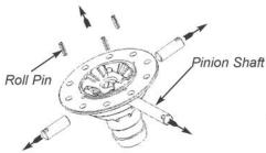
14. Remove roll pins and pinion shafts.
