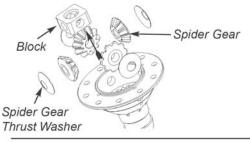
15. Remove spider gears, spider gear thrust washers, and block.
