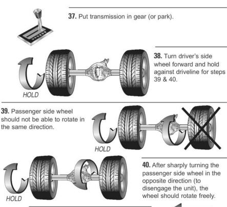
**41.** Repeat the test for both wheels in both directions.
