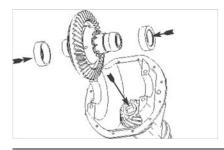
**33.** Reinstall each bearing race *on its original bearing* and install the assembly in the third member.
