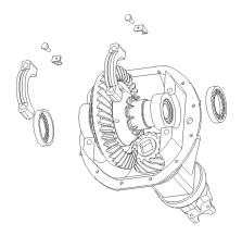
**9.** Remove adjuster locks, bearing caps, and bearing adjusters from the third member. *These parts should have been marked in Step 8 as they are not interchangeable and must be reinstalled in their original positions.*
