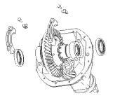
**34.** Reinstall the bearing caps *in their original positions.* Install the bearing adjusters back *in their original positions.* Tighten bearing caps down to required torque and reinstall bearing adjuster locks.
