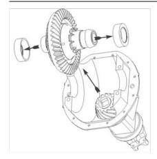
**10.** Pull out the differential case from the third member. Remove the bearing races from the bearings and mark them. *The bearing races must be reinstalled on the same bearings they were originally on to avoid bearing failure.*  **11.** Mark the position of the ring gear to the two halves of the differential case and remove the ring gear. *The ring gear must be reinstalled in its original position.*
