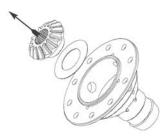
16. Remove the second sidegear and thrust washer.
