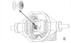
**11.** Remove remaining side gear and thrust washer.
