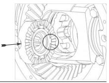
**24.** Verify spacer paddle is aligned with the paddle opening in synchro ring and press down on driver /spacer to seat on coupler; driver teeth should be fully engaged all the way around.
