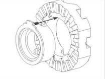
**19.** Insert driver/spacer as shown, making sure spacer paddle is facing out towards you.
