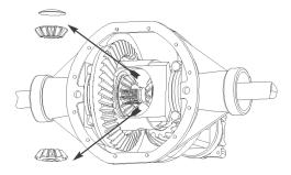
**9.** Remove both spider gears and their thrust washers.
