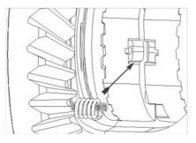
**31.** Visually inspect notches in spring slot to make sure inner spring is fully seated.
