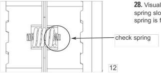
**28.** Visually inspect notches in spring slot to make sure inner spring is fully seated.
