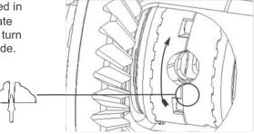
**30.** Compress inner spring and install the second spring assembly into the second spring slot.
