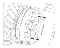
**20.** Verify spacer paddle is aligned with paddle opening in synchro ring and press driver/spacer down onto coupler. Driver teeth should be fully engaged all the way around.
