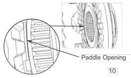
**22.** Verify paddle opening (widest gap) in other synchro ring is facing the back of the differential, away from you.
