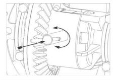
**37.** Insert retaining bolt/roll-pin into case/shaft.
