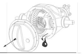
**7.** Expose pinion shaft; remove retaining pin/roll pin. Remove pinion shaft.
