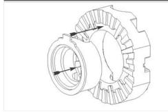
**21.** Insert the second active spacer into the second driver. Seat the spacer paddle at the missing extended tooth.
