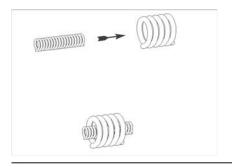
**26.** Place the two inner springs inside the two outer springs.
