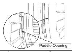
**18.** Insert an active spacer into a driver. Seat the spacer paddle at the missing extended tooth.
