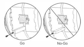
**32.** Check the gap between drivers using check block. The narrow side of the block should fit inbetween drivers, but the wider side should not fit.
