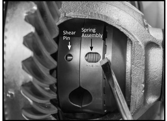
Figure 8: Snap spring assembly into hole
