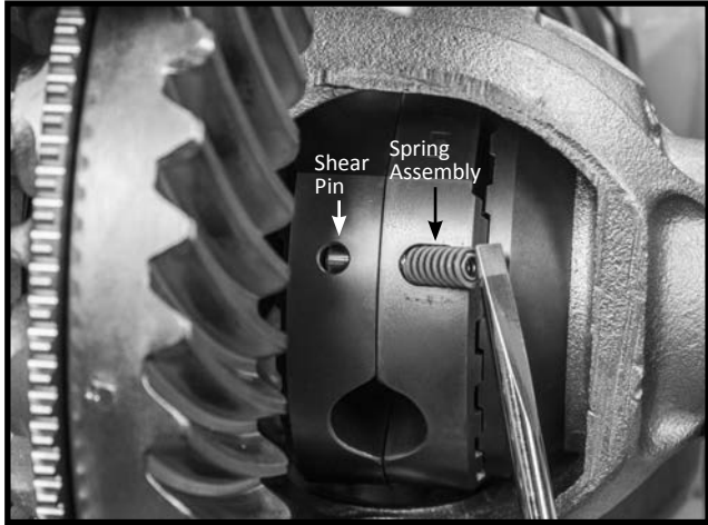
Figure 7: Install spring assemblies in holes
