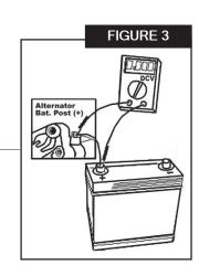
♦ With battery fully charged and engine running at 1,500rpm, measure the voltage at battery positive post (+) and the ground post (-). Voltage should be 13.8~14.5VDC. Readings above 15.5VDC indicate a defective alternator and readings below 12.7VDC indicate that the alternator is not functioning or cannot supply the present amperage needs of the vehicle at this engine speed.
