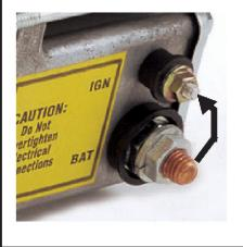
2. Connect the positive battery wire to the "BAT" terminal on the starter solenoid.
