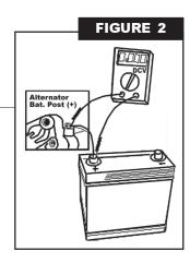
indicate a defective alternator and readings below 12.7VDC indicate that the alternator is not functioning or cannot supply the current amperage needs of the vehicle at this engine speed.
