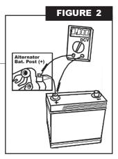
♦ Using the voltmeter, measure the voltage drop between the batty positive post (+) and the alternator output post (See figure 2). Voltage should be less that 0.40VDC. If voltage is higher that 0.40VDC, check for poor connections between the alternator and the battery. Possible causes are unsized battery cables, loose or improperly crimped terminals, and corroded connections.
