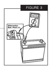
indicate a defective alternator and readings below 12.7VDC indicate that the alternator is not functioning or cannot supply the current amperage needs of the vehicle at this engine speed.
