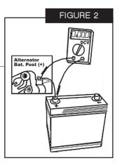
♦ Using the voltmeter, measure the voltage drop between the batty positive post (+) and the alternator output post (See figure 2). Voltage should be less that 0.40VDC. If voltage is higher that 0.40VDC, check for poor connections between the alternator and the battery. Possible causes are unsized battery cables, loose or improperly crimped terminals, and corroded connections.
