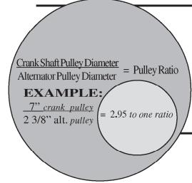
To calculate a vehicle's pulley ratio, the engine's crank pulley diameter should be divided by the alternator's pulley diameter. This ratio should then be multiplied times the highest expected engine RPMs. The result will be that vehicle's maximum alternator RPM.
