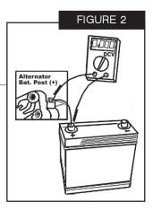
♦ Using the voltmeter, measure the voltage drop between the batty positive post (+) and the alternator output post (See figure 2). Voltage should be less that 0.40VDC. If voltage is higher that 0.40VDC, check for poor connections between the alternator and the battery. Possible causes are undersized battery cables, loose or improperly crimped terminals, and corroded connections.
