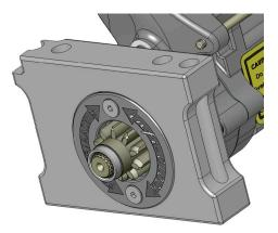
Using Blue Loctite® or equivalent thread lock on the two ring bolts is REQUIRED!
