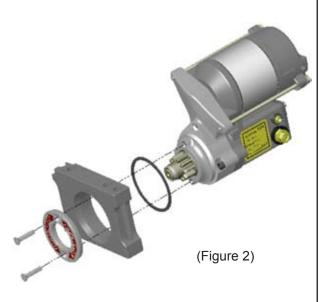
\*Powermaster recommends no more than one set of internal shims be installed in a starter.
