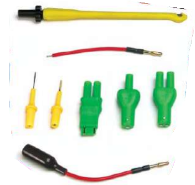
Fig.1 There are times when a short or open circuit is located closer to the tail light or brake light circuit. It is here where you may find it much easier to diagnose the circuit by injecting a signal into the light socket directly. The bulb socket adapters provide a quick and easy way to connect to bulb socket terminals.
