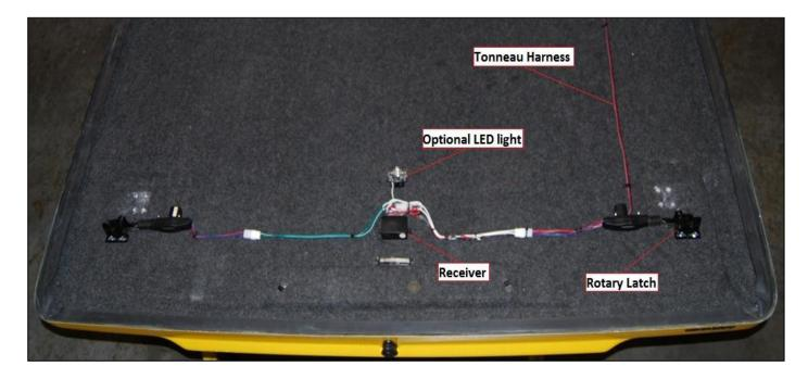
3) Connect receiver actuator outputs to the actuators and bundle up and wire tie any excess wire length.
