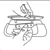
Lift the handle assembly out and remove the mounting bracket located under the handle.
