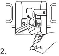
Unscrew the two nuts using a 10MM wrench holding the handle assembly. DO NOT CLOSE TAILGATE FROM THIS POINT ON.
