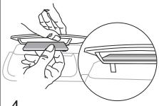
Clean the inside of the handle with the alcohol wipe and attach the striker plate to the interior rear wall with the double-sided tape as shown.
