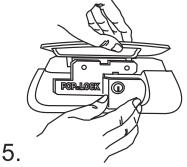
Insert the Pop&Lock assembly in place of the mounting bracket.
