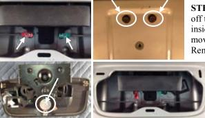
**STEP 2** - Remove the latch rods from the latch rod clips. Do this by turning the clip off the rod and pulling the rod out of the clip. Remove the other two bolts on the inside (backside) of the tailgate. Hold the handle at the same time to keep it from moving as you remove the bolts. Next remove the OEM handle from the tailgate. Remove the bolt that holds the Pop N Lock components together (do not discard the
