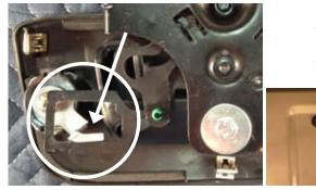
**STEP 3** - Insert the latch rods into the rod clips and snap the clips onto the rods. Install the Pop N Lock lock bezel. Make sure the lock arm aligns to go into the square opening on the handle assemble. Snap the bezel clips into the tailgate. Place the bolt and washer (was removed to separate the components) into the bottom center hole on the
