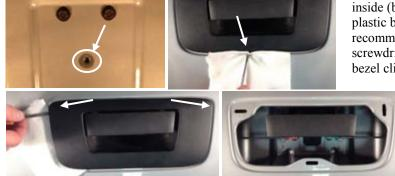
**STEP 1** - Lower tailgate and remove the bottom center bolt on the inside (backside) of the tailgate. Gently shut the tailgate. Remove the plastic bezel by carefully prying with a flat head screw driver (it is recommended to use a rag or cardboard between the tailgate and screwdriver so not scratch the paint) in the bottom center to pop the bezel clip out of the tailgate. Next gently pry at the upper two corners
