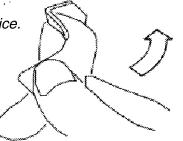
Tighten an adjustable wrench over the tip of the cam and bend it 10 - 30 degrees to provide more clearance.
